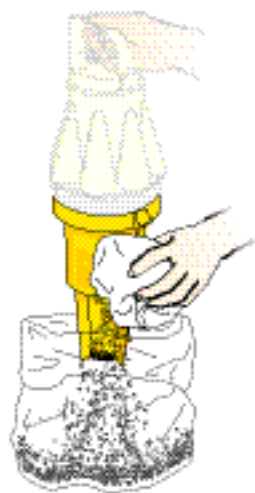
UK. Press catch 3 to release bin. Remove fine dust with a cloth or small brush.
